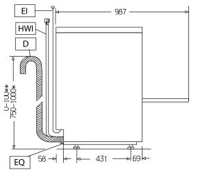
EI Electrical inlet (power) Electrical Outlet
